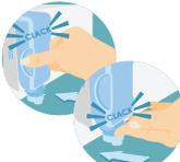
4 Insert the tank into its **designated bay** and push until you feel it click into place. Check the correct coupling by applying **pressure on the neck**.
