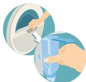
2 Open the detergent compartment **door**. If present, **remove** the exhausted tank you wish to replace by squeezing the knurled areas on the sides, then pulling outwards.
